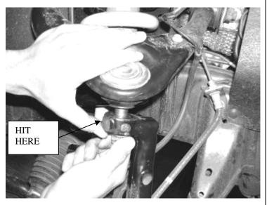
3. Loosen the tie rod nut. Using the appropriate tool to remove the tie rod end. Save all hardware (Use care not to damage threads.) Disconnect the factory swaybar endlinks and save with the hardware. SEE PHOTO BELOW.
