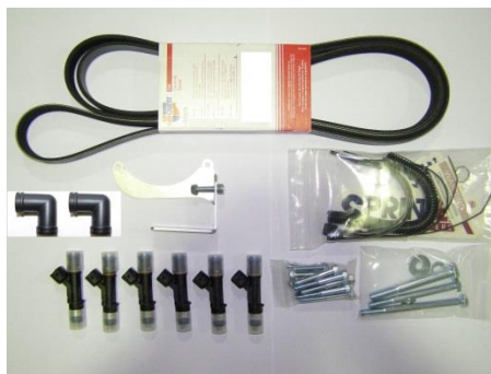
Drive belt, Fuel injectors and ancillary parts
